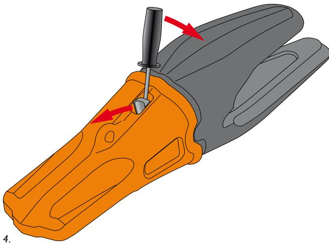
4. Push the securing part forward to release the tap from the tooth.
