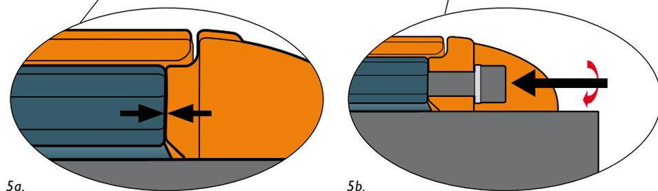
5. Put the bolt protector in place and tighten the screw to recommended torque in Table G.
