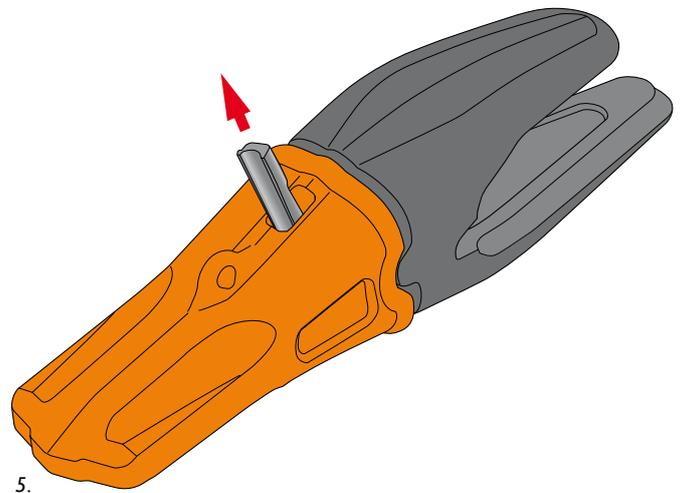
5. Lift the securing part and remove the lock.
