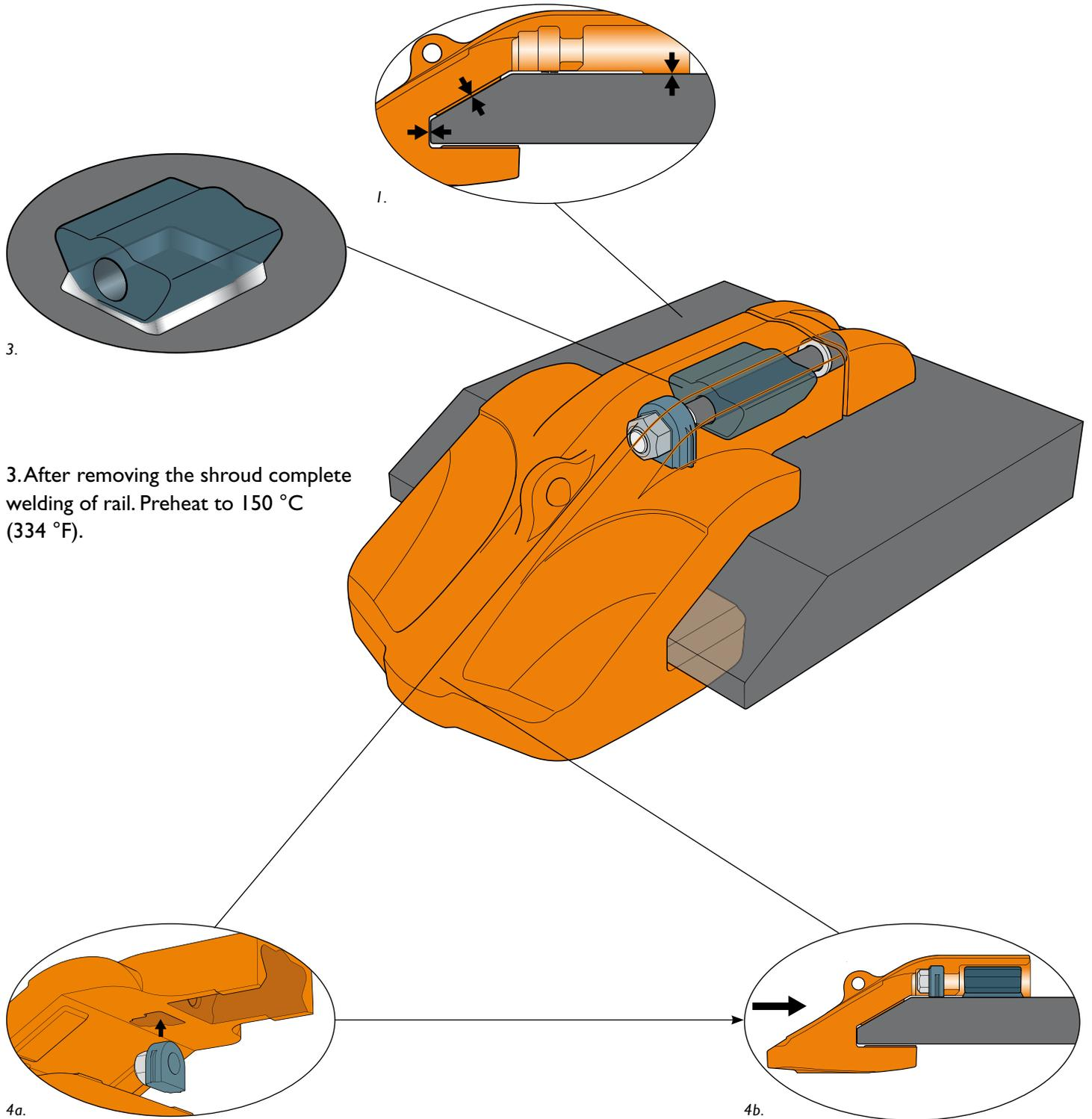
3. After removing the shroud complete welding of rail. Preheat to 150 °C (334 °F).
