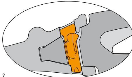
2. Tap the lock into place with a sledge hammer. When in place the lock is embedded in the tooth.
