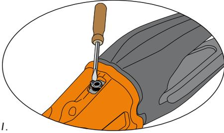
1. Remove the rubber hat. Clean from dirt around the head of the screw.
