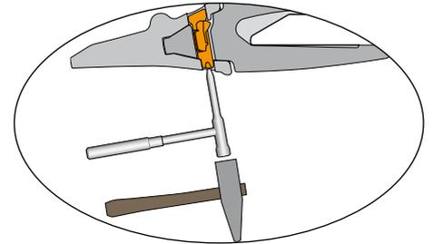
The lock is dismounted from the bottom. Place the dismounting tool in the recess in the lock. Tap the lock until it can be removed by hand.
