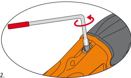
2. Unscrew and remove the screw.
