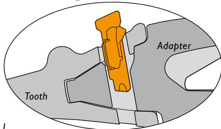
1. The lock shall be mounted with the securing part facing into the bucket. The locking device can be mounted half-way by hand. At this point the tooth is securely attached to the adapter.
