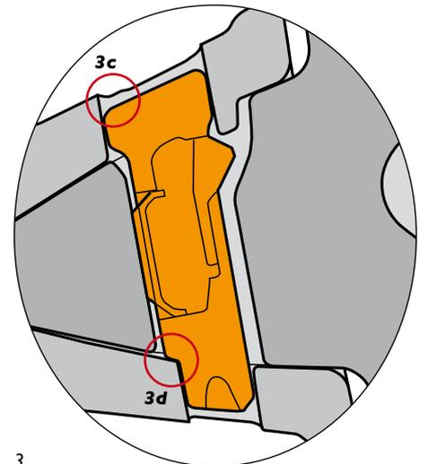
3. When lock is correctly mounted the lock should sit below the surface of the tooth (3c) and in (3d) contact at the bottom stop surface.
